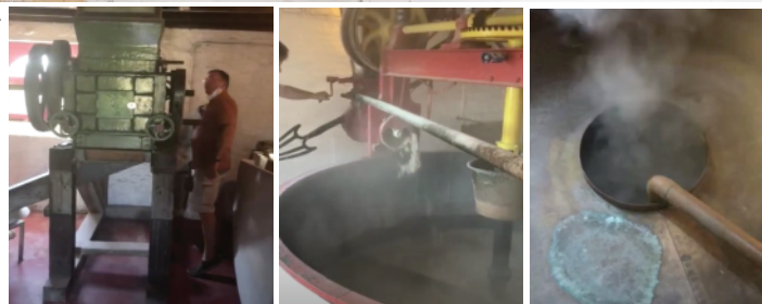
(1) Simpson Maris Otter Pale-Ale malt has to be blownd and crushed upstairs - the crusher is original from 1921, the restart after WWI (2) Brewing starts with mashing - the copper brew house dates from 1921 (3) Boiling for a couple of hours and addition of flower hops - Whitbread Golden Variety
